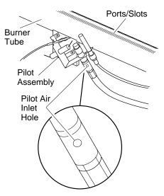
Figure 27 - Pilot Inlet Air Hole
